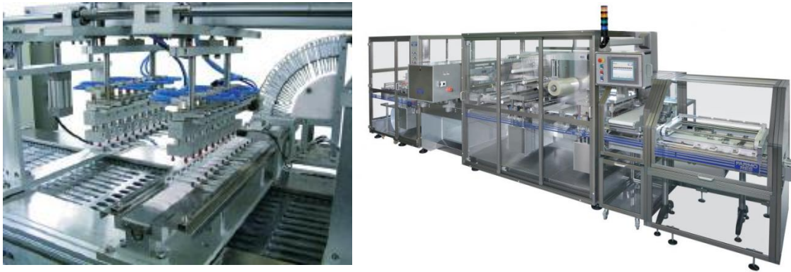
Figure 15-12. Left: internal view of a blister packaging machine (courtesy Greathealth Trexim) Right: tray pack thermoforming machine (courtesy MG America)
