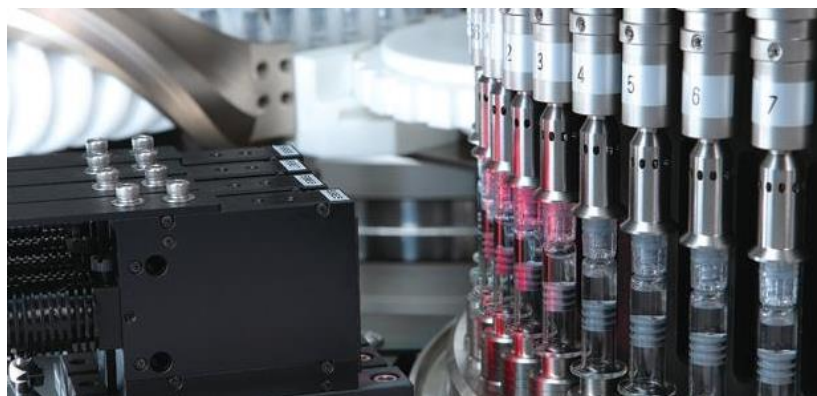
Figure 15-4. Automated syringe inspection using optical sensor to detect particulates (courtesy Eisai Machinery and Bosch Packaging Technology)
