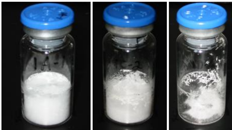
Figure 9-7. Examples of visual inspection: Fully intact cake, broken cake, and collapsed cake
