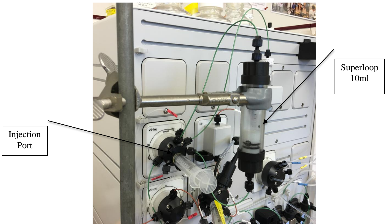
Fig. 4. Detail of Injection Port with Syringe in Place.
