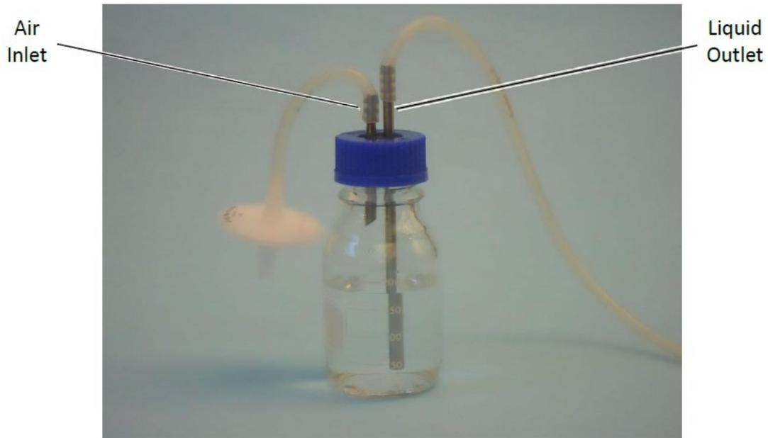
Figure 7. Liquid Addition Bottle
