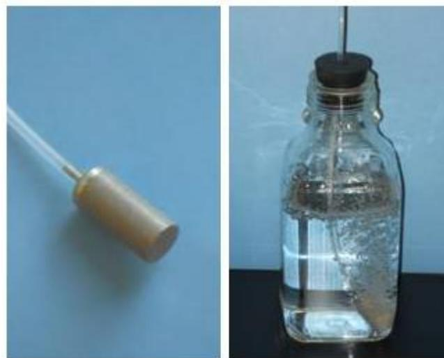
Figure 2. Porous Metal Sparger
