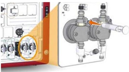
Starting with B1, attach a 10 ml syringe to the pump priming fitting and open the valve one full turn or more until you are easily able to withdraw 10 ml of liquid, which will insure the line is full of liquid and any bubbles are out of the line. Repeat these steps to prime every pump. Note that you will need to use the System Control window to manually switch A1 to A2 and
