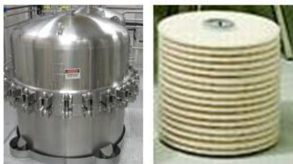
Figure 10-34. A depth filter housing and internal filter stack
