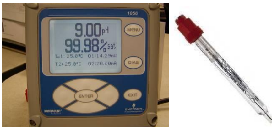
Figure 10-12. Combination Dissolved Oxygen (DO) and pH probe transmitter
