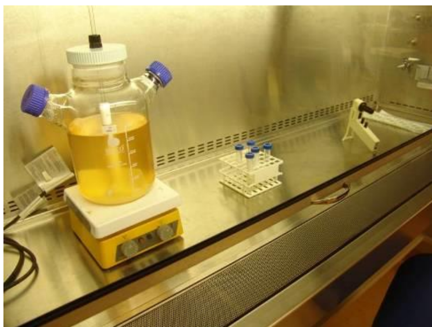
Figure 10-6. Spinner bottle containing cells and media on spinner plate within a Biosafety Cabinet
