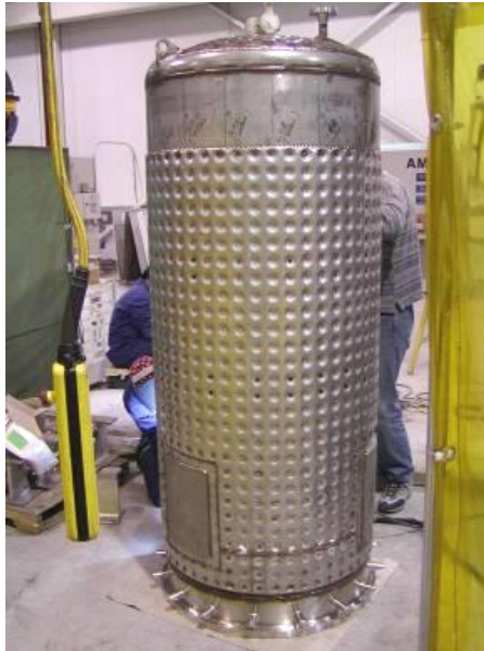
Figure 10-19. Dimpled surface of the bioreactor jacket (interior view of jacket)
