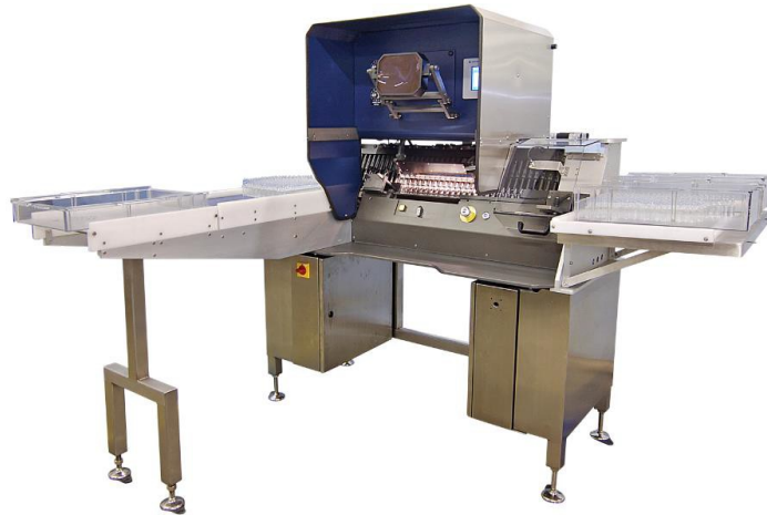
Figure 15-2. Pharmaceutical semi-automatic inspection booth (courtesy Dabrico, Inc.)
