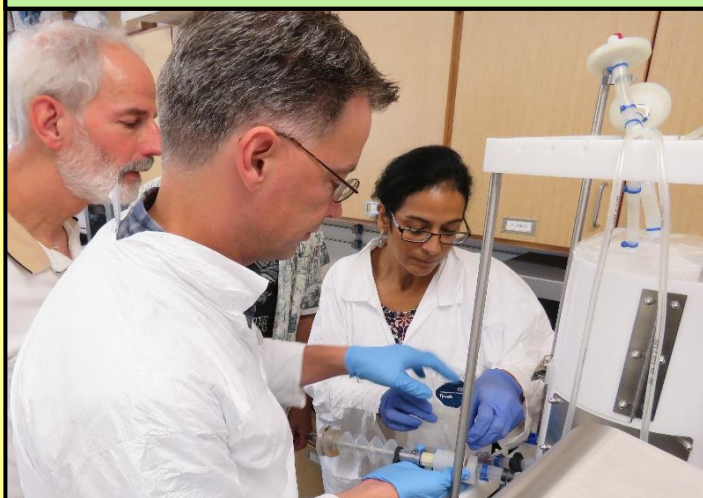
miniBIOMAN participants learn to aseptically sample cultures of mAb producing CHO cells (above) and set up pH and DO probes into a 10 liter single-use bioreactor (below)
