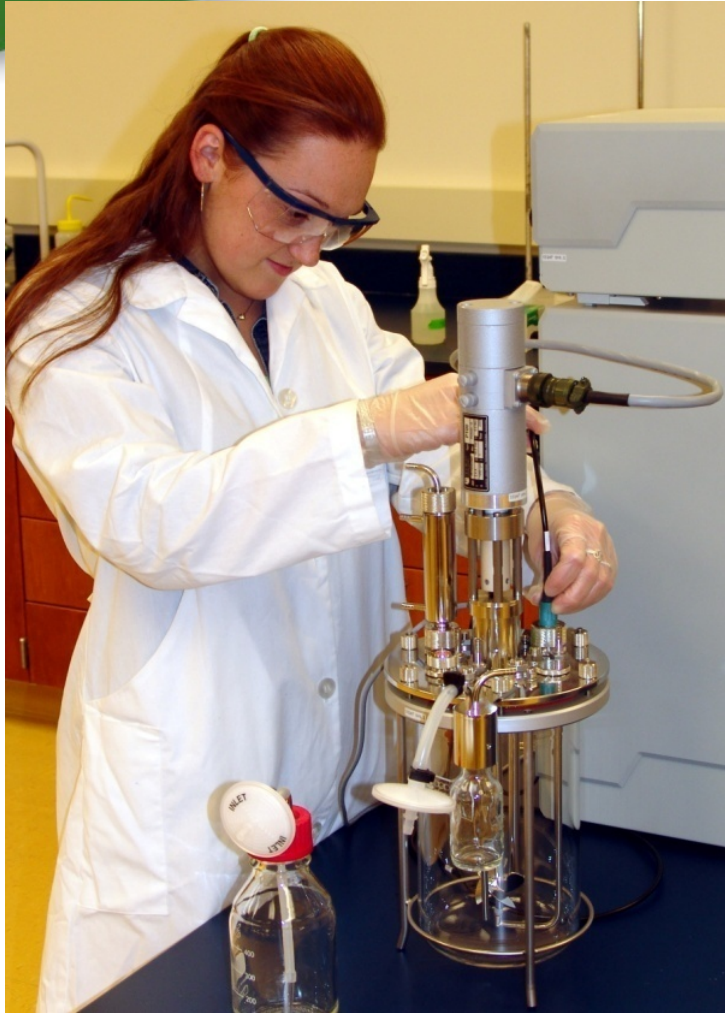
Lab-Scale Bioreactor 3 liters
