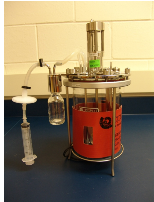
Heating Blanket on single wall vessel
