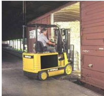
Figure 5-16. Forklifts are used to move materials from off-loading points to warehouses.
