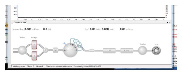
Now, if you click on each component you will see functions or parameters that you can change manually (via the software). For example, clicking the Inlets depicted (on the left side) allows you to switch the A inlet line and pumps between A1 and A2. Similarly you can switch between B1 and B2.
