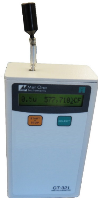
Figure 8-9. Non-viable portable particle counter displaying real-time test results
