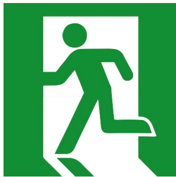
Sign Marking Exit Route
