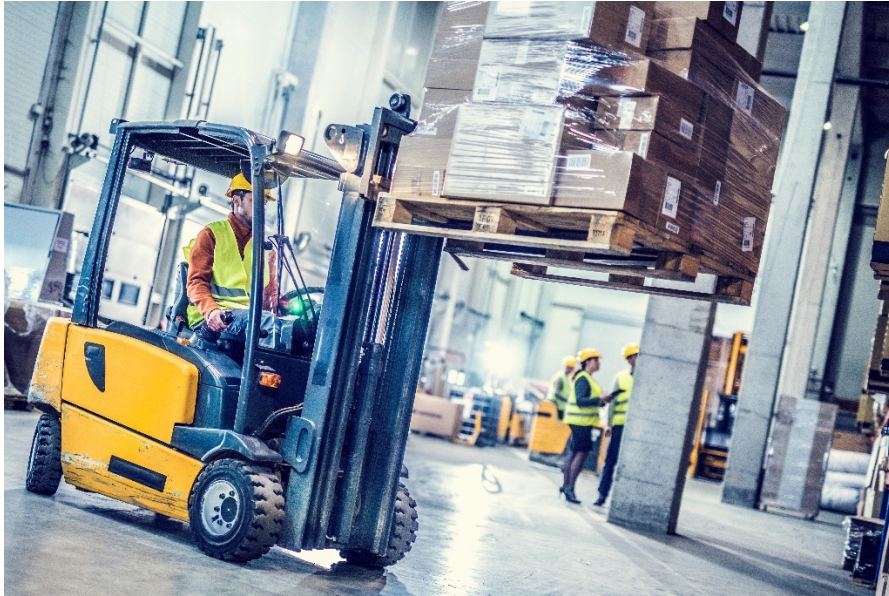
Figure 5-15. Forklifts are used to move materials from off-loading points to warehouses.
