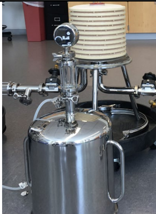
Figure 10-25 A depth filter housing and internal filter stack
