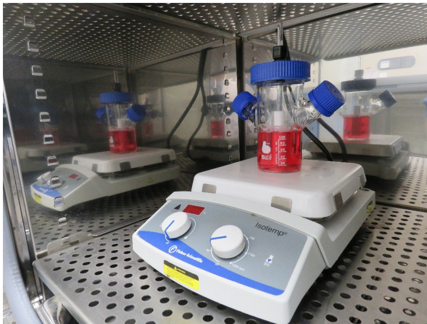
Figure 10-4. Spinner bottle containing cells and media on spinner plate within an incubator
