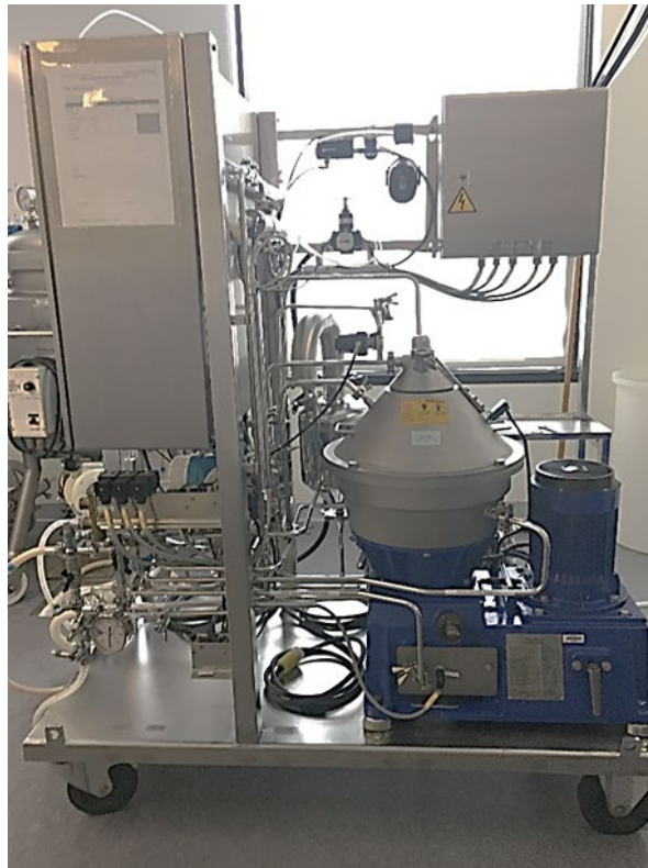
Figure 10-24. A centrifuge, motor and associated piping
