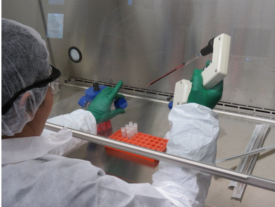
Figure 10-3. Aseptic preparation of cell bank vials in a Biological Safety Cabinet (BSC)
