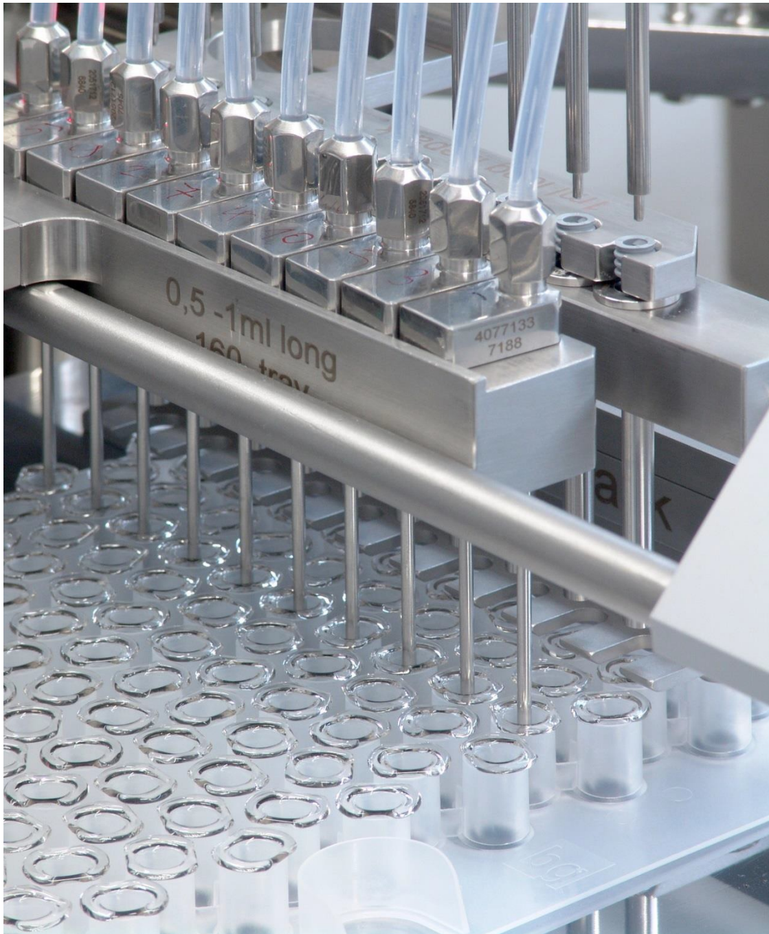
Figure 14-18. Inova syringe filling machine needle and plunger assemblies (courtesy OPTIMA Corporation)
