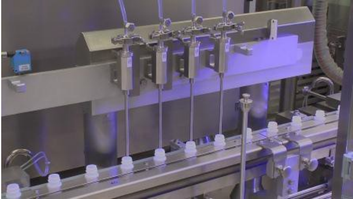
Figure 14-16. Inova vial filling machine with time pressure pumps and in-line check weighing (courtesy OPTIMA Corporation)
