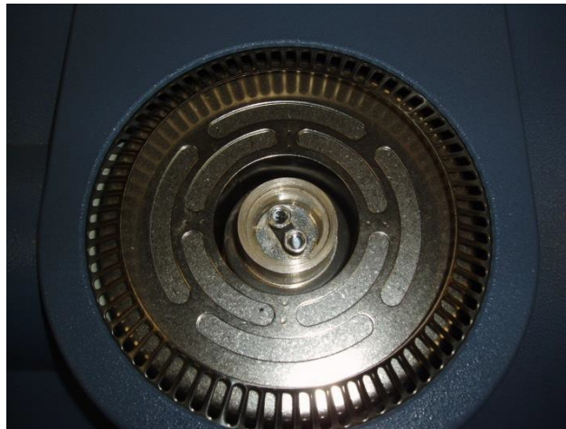
Figure 14-37. DSC sample and reference furnaces (courtesy/permission TA Instruments)
