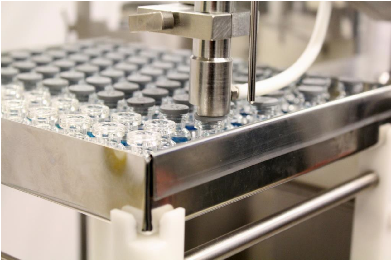
Figure 14-19. Vial filling system depicting stoppering process (courtesy Colanar)
