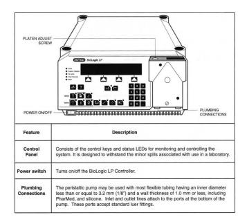
Figure 1: Controller Front Panel
