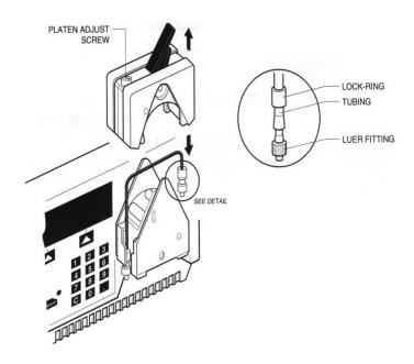
**Figure 2: Controller Pump**
