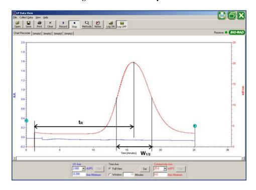
Figure 5: Chromatogram Example for Calculating HETP
