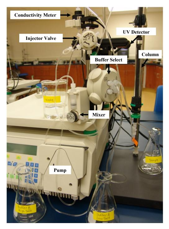
Figure 3: LP Biologic System Parts
