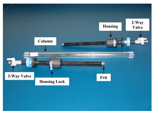
**Figure 4: Column Components**
