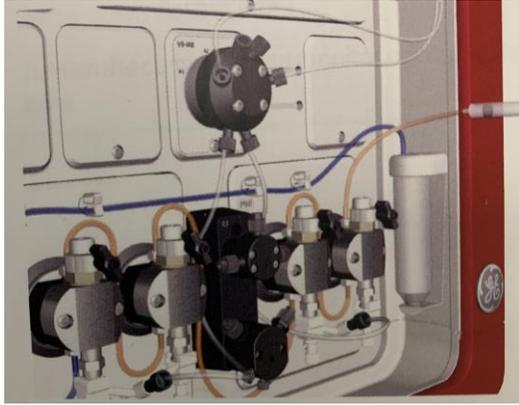
(Note: Make sure that the inlet tubing reaches close to the bottom of the rinsing solution tube)
