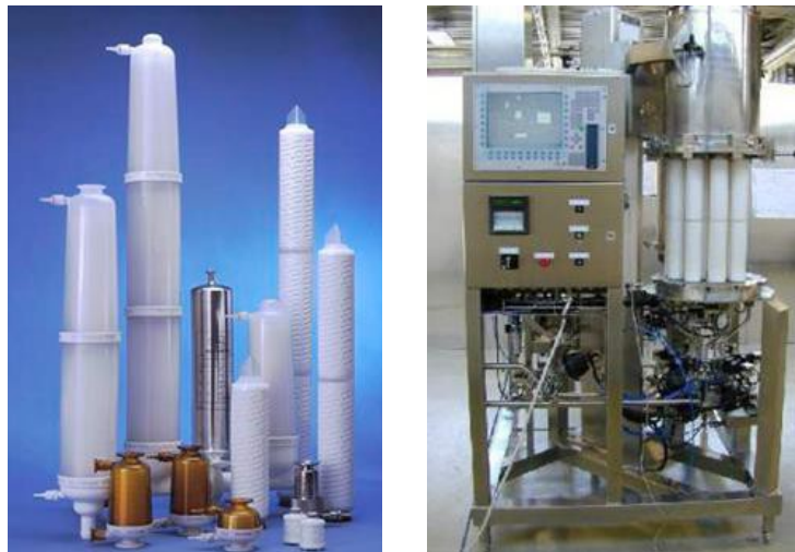
Figure 11-2. Pall Life Sciences Ultipor® Direct Flow Filtration (DFF) cartridges of various scales (top) and typical automated process DFF system fitted with a multi-round assembly of cartridges in a single housing—partially lifted from its base to expose the cartridges (bottom)—courtesy Pall Life Sciences
