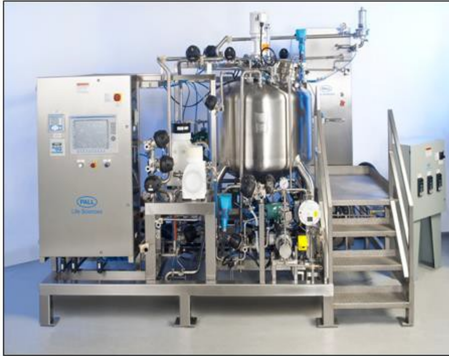
Figure 11-14. Integrated system for packing and qualifying a chromatography column of 80–100 cm diameter—approx. 50–150 liter scale (courtesy Pall Life Sciences)
