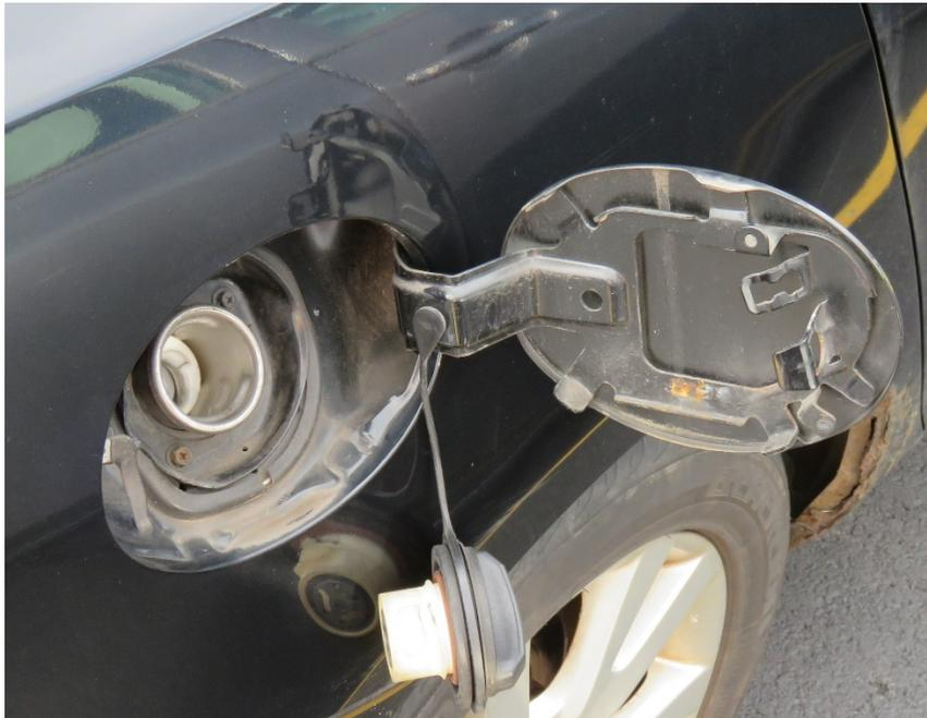
**Figure 6-12. Example of an error-proofing device: a gas cap strap**
