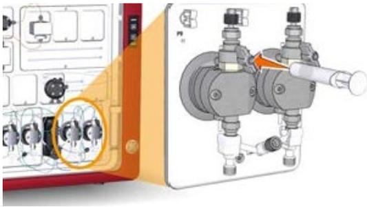
Starting with B1, attach a 10 ml syringe to the pump priming fitting and open the valve one full turn or more until you are easily able to withdraw 10 ml of liquid, which will insure the line is full of liquid and any bubbles are out of the line. Repeat these steps to prime every pump. Note that you will need to use the System Control window to manually switch A1 to A2 and
